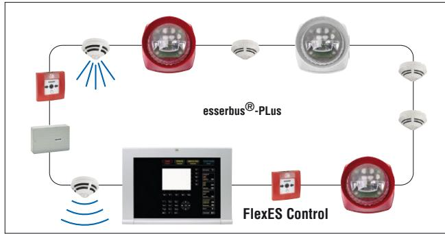
IQ8Alarm Plus connected to the esserbus-PLus at the FACP FlexES Control.
