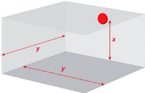
x = maximum mounting height on the wall ( $\geq 2,4$  m)
